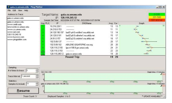
Next, send a set of datagrams with a longer length, by selecting *Edit->Advanced Options->Packet Options* and enter a value of 2000 in the *Packet Size* field and then press OK. Then press the Resume button.
