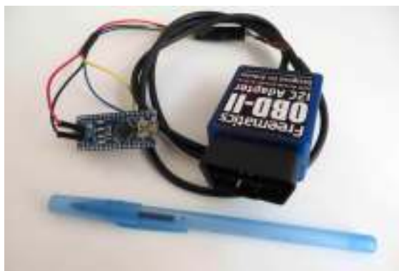
Figure 3. Privacy-preserving driving data aggregator device prototype.
